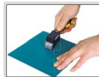
step 1: make grid cutting on surface
